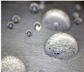
Using hydrophobes like the ENVIROGUARD WR series physically repels water keeping treated surfaces dry, keeping acid gases out.
