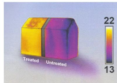
Therefore using the ENVIROGUARD WR series of hydrophobes to keep surfaces dry, reduces thermal conductivity and increases energy efficiency.
